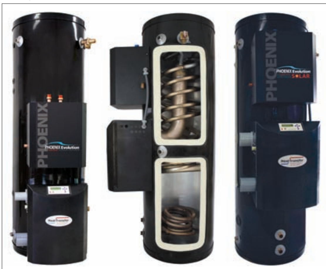
The Phoenix Evolution includes four distinct components, each of which contributes to its efficiency: A modulating condensing gas water heater for DHW, an attached heating module that draws heat directly from the hot water to supply space heating, auxiliary ports for air handlers or additional storage, and an optional solar heat exchanger.
