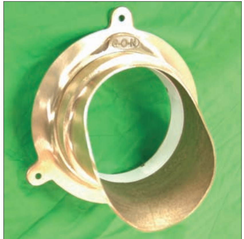
With the Glue-On-Nozzle the plumber simply stubs-out the pipe, then trims the stub to length after the wall is finished and attaches the nozzle with cement.
