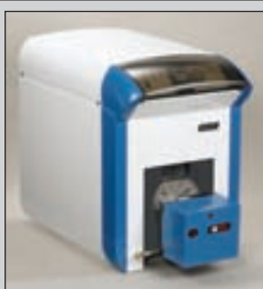
The specially designed three-pass heat exchanger maximizes heat transfer and delivers 87% AFUE. Plenty of room for thermal expansion of the flue gasses to keep burner and flame noise to a minimum.
