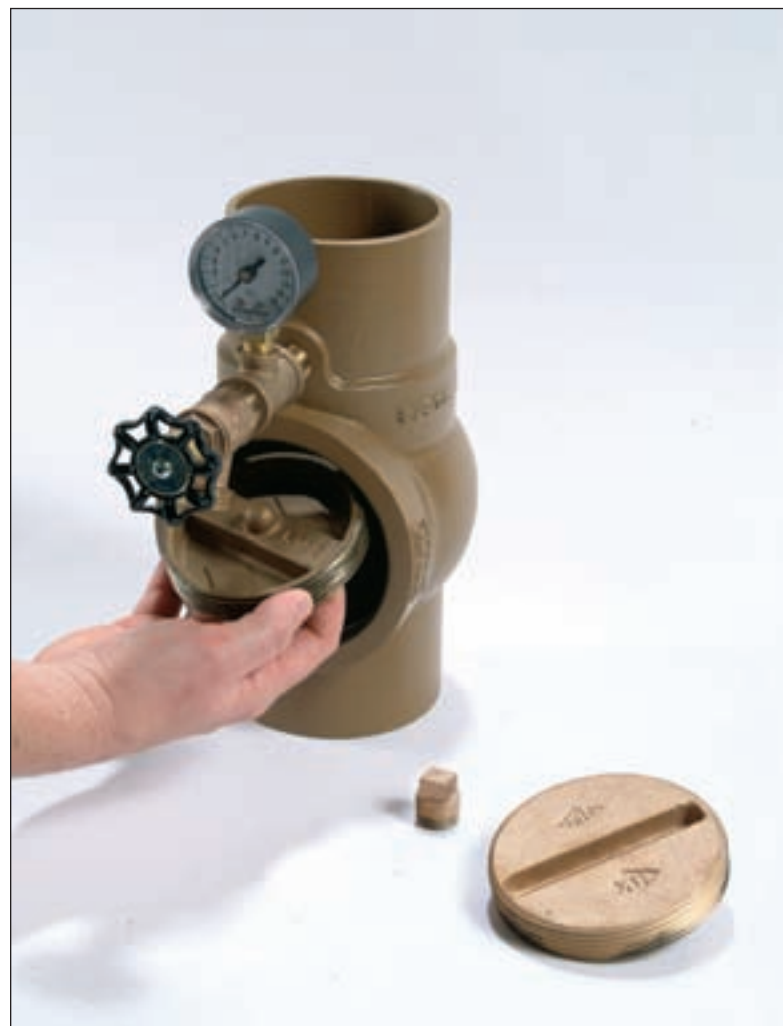
The Boss Tee, figure number 4505 does two jobs in a DWV piping system: 1) During construction it is used to hydrostatically test up to three floors of the piping system; and 2) after testing it serves as a standard cleanout tee.
