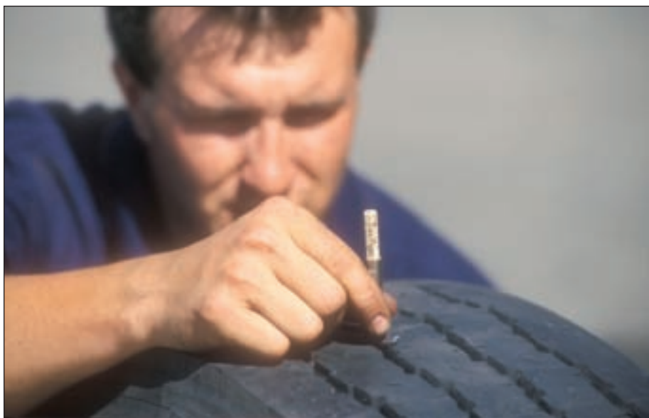
Measuring tire tread for wear is only part of proper tire maintenance. Matching tire wear and circumference between duals and across axles is another aspect of getting the most out of your tires.
