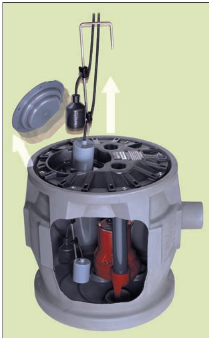
With QuickTree® technology, the floats are mounted to a stainless steel tree (or rod) underneath a separate access cover. Floats can be replaced or cleaned by simply removing the cover and lifting the tree from the unit.
