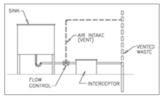
Figure 5 – Typical grease interceptor serving a single sink with a vented flow control device.
