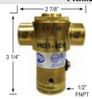
The **Prime-Pro™** is activated when sensing potable water flowing at an adjacent plumbing fixture. This trap priming device must be installed on the cold water line leading to the plumbing fixture; the valve then emits fresh cold potable water to a floor drain trap as long as the fixture is in use, providing adequate trap seal. Providing potable water to the trap seal is essential in preventing sewer gas escape and bacteria growth.
