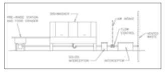
Figure 6 – Typical grease interceptor that serves a dishwasher and pre-wash sink with a disposer and solids interceptor.
