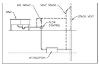
Figure 2 – Two-compartment sink with a vented flow control orifice on the same level as the sink and the grease interceptor on the floor below.
