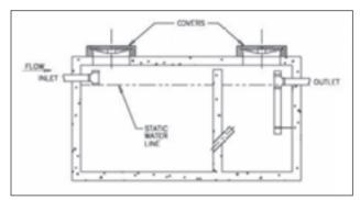
Figure 3 – Typical gravity grease interceptor.
