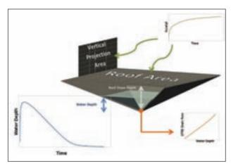
Figure 1 CFRD Dynamics: Rainwater enters the roof simultaneously as water drains through the CFRD. The difference between water inflow and outflow results in a water depth that initially increases, peaks and then decreases as rainfall intensity weakens. Note that the roof slope depth has been exaggerated in this figure to illustrate the inverted rectangular pyramid structure of the roof.
