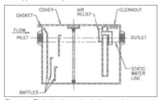
Figure 1 – Typical hydro-mechanical grease interceptor.
