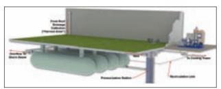
The disinfection and treatment station filters, disinfects, recirculates, colorizes and stores the water under pressure, ready for its intended use.
