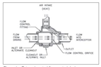
Figure 4 – External vented flow control device.
