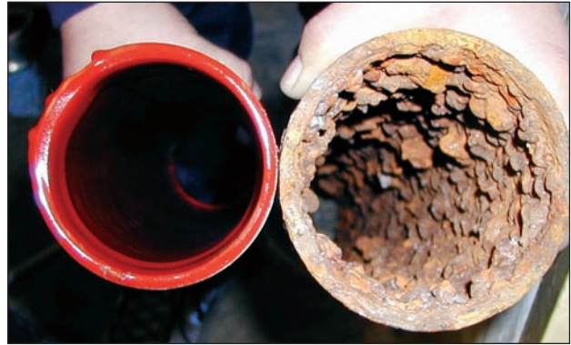
Pipe lining prevents toxic heavy metals from leaching into drinking water and prevents leaks and breaks. Each year, leaks cause billions of dollars in water damage.
