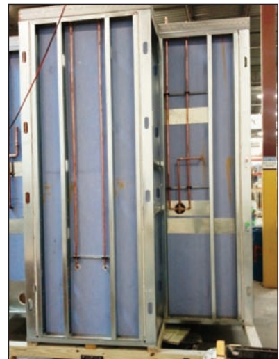
Fig. 2: Rear side of a PIVOTek toilet module, piping exposed but not yet insulated.
