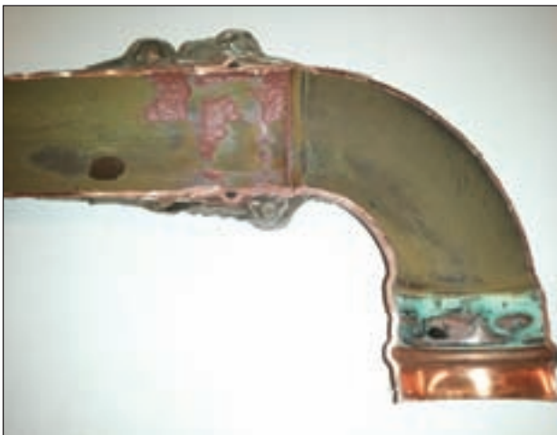
Figure 1: Erosion-corrosion in hot water circulation piping
