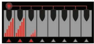
On-board cascade connects up to eight boilers for coordinated operation. Built-in multiple boiler control improves system efficiency, reducing operating costs.
